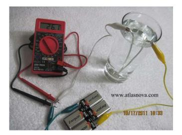
In order to speed up the process you can move the silver wires closer together so that you may generate ions more quickly. The more ions in the water, the higher the conductivity of the water and this allows more current to flow.
