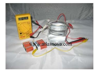
The voltage reading of 4.3 volts across the resistor indicates a current of less than 0.1 milliamps. This is the maximum amount that is allowable in terms of how good your distilled water is. If it reads much more than this you need to find a better source of distilled water.
