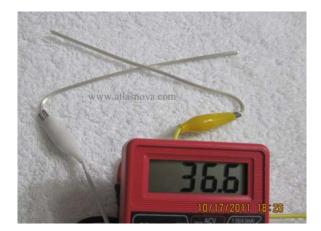
When you put the two silver wires together, this causes the full voltage to flow through the resistor and the meter will read approximately thirty six volts, which happens to be four times nine.
