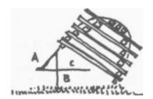
PLATE 224 Diagram shows scale of the sticks used to make the trigger. Stick "A" is 9" long, "B" is 9/2", and "C" is 20". The sticks are the same as those used for the deadfall trap (see PLATE 229).
