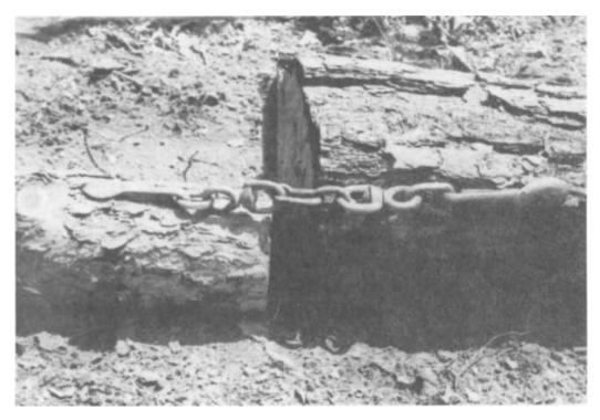
PLATE 265 In order to drag several logs out of the woods together instead of having to drag each separately, the logs are hooked together with "trailer grabs"—metal hooks connected by swivel links so the logs can turn independently—and two links of chain.
