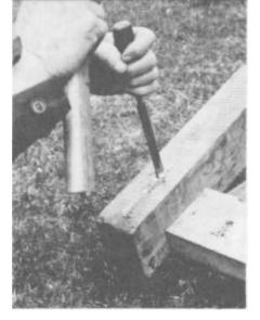
PLATE 169 After the bottoms of the pegs are sawed off flush, Tedra splits the bottom of each peg. Then he drives a wedge into the split to make the peg bind firmly in the hole.
