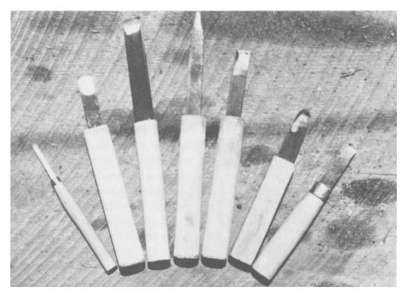
PLATE 126 His set of homemade chisels, many made of old files.
