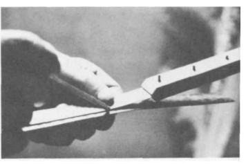
PLATE 13 Then, using another knife blade as a pattern, he marks the width of the blade on the new stock.
