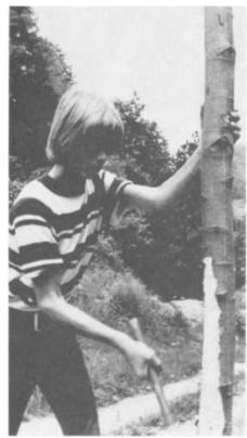
PLATE 173 On our second visit, we added the half soles to the runners. Here, Ken Cronic hews two green poplar poles so each has a flat side. Normally the half soles would be of white hickory for longer life.
