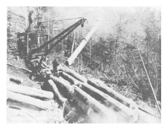
PLATE 278 A "stiff-necked" loader at work. The loaders were steam powered, and their boilers were often called "coffeepot boilers." (Photo courtesy of Champion Paper.)
