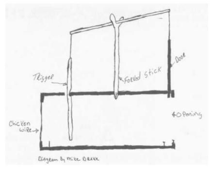
PLATE 234 Diagram illustrates the trap mechanism.
