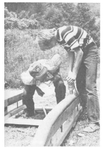
PLATE 179 Ken drills holes at regular intervals (four holes per half sole, in this case) for the pegs that will pin the half sole into place.
