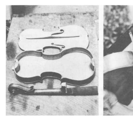
PLATE 137 The top is ready to be glued to the back and sides. Note the blocks at either end of the back to which the sides are glued, the double lining, and the triangular support blocks where the sides come together in the middle.
