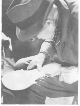
PLATE 113 With the plane, Harley shapes out the top and the back of the fiddle until they are about 1/8" thick.
