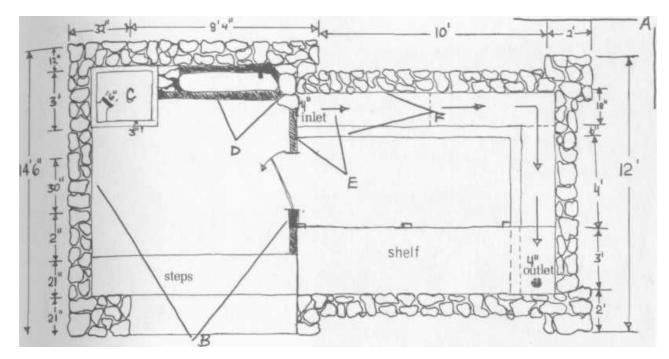
PLATE 333 Diagram of the Hambidge springhouse.
