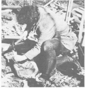
PLATE 108 He also shapes the bowl by using a hammer and chisel as he begins to get closer and closer to the critical points. Here, Roy Dickerson, the author of this chapter, tries his hand at it.
