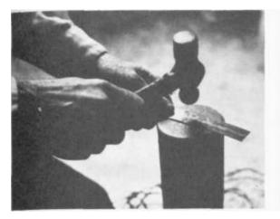
PLATE 12 Now, using a ball pecn hammer, he pecks the steel until the curve is removed and it lies flat.
