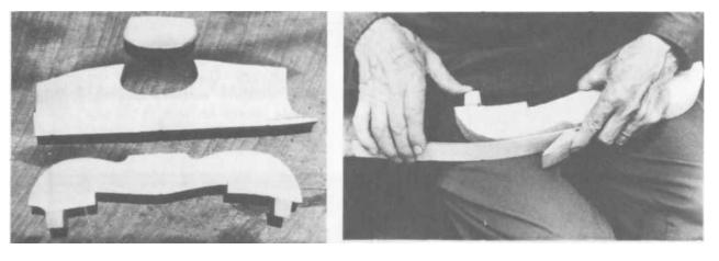
PLATES 133-134 The sides are clamped into forms as shown.
