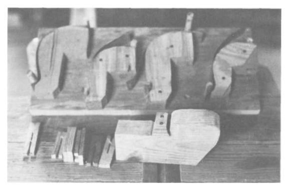
PLATE 115 The "'ribs' or sides of the fiddle arc thin strips of maple  $1 \frac{1}{4}$ " wide, and arc soaked in hot water until pliable and then placed in wooden forms to harden in the correct shape. Blocks of maple 1  $\frac{1}{4}$ "-high are placed at each end of the top to hold the ribs secure (see Plate 120),
