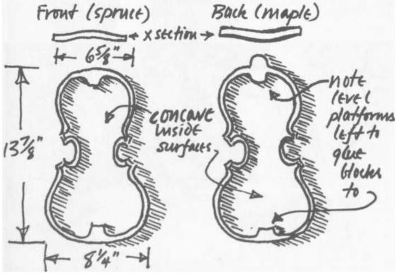
PLATE 112 The patterns used for the fiddle's top and back. These are each made of two pieces of wood 5/8"X 15"X4 1/4" that are glued side by side lengthwise with Elmer's Glue. (The fiddle is held together only by glue.) The top is made of spruce to produce the be\* sound. All other parts are made of maple (curly maple is host) except the finger board, which is ebony. The diagrams indicate how the top and back should be shaped, and the areas to be "dug out".
