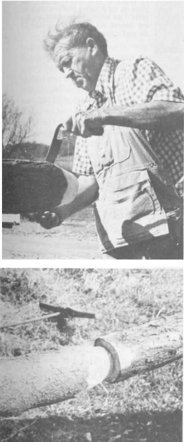
PLATE 312 When the pipe is drilled, he uses a drawknife to taper one end.
