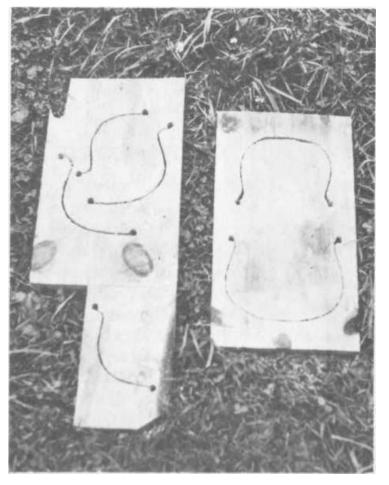
PLATE 144 The forms that Clarence uses to shape the sides or "ribs."
