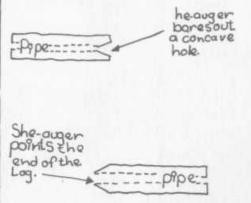
PLATE 313 He then takes another auger and bores a concave hole in the other end of the pipe.
