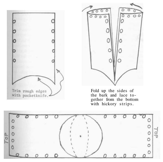
The slit for the bottom of the bucket may be circular or oval.
